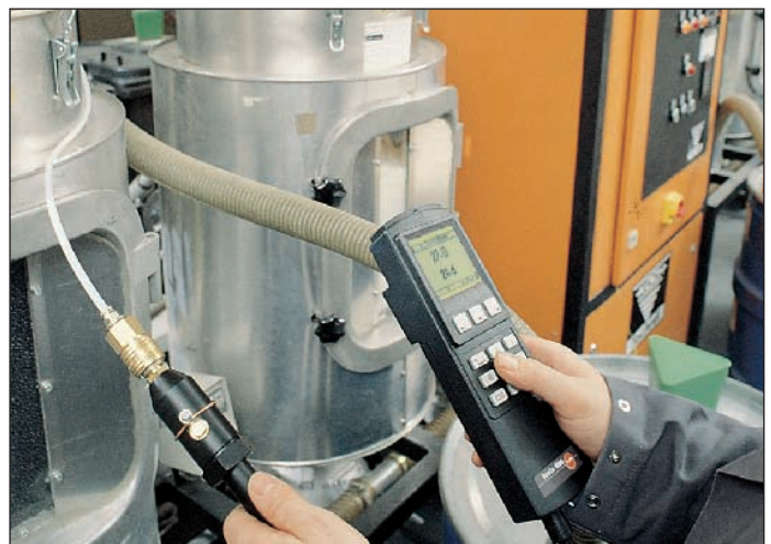
Pressure-tight precision probe for measuring the remaining moisture in compressed air systems, plastics driers... Advantage: display in g/kg, g/m 3 , pressure dew point
