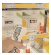
A limit value set by the user is monitored during the measurement. An audible alarm sounds when this limit is exceeded, and "Alarm" appears in the display.
