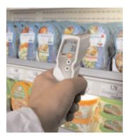
During temperature checks in refrigerated displays, the 2-point laser shows the position and size of the measurement point exactly.
