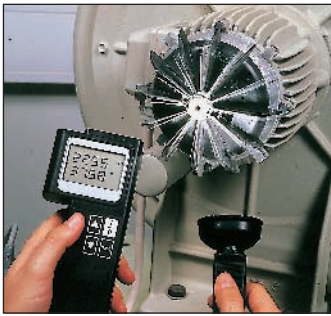
Measures the rpm of fans, motors, rollers etc., without reflectors
