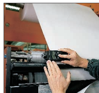
Mechanical rpm measurement on a roller
