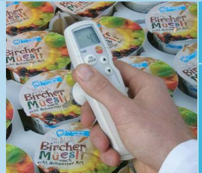
Exact measurements on arrival of the product with alarm if limits are exceeded
