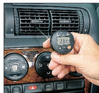
Measurements on air conditioning systems
