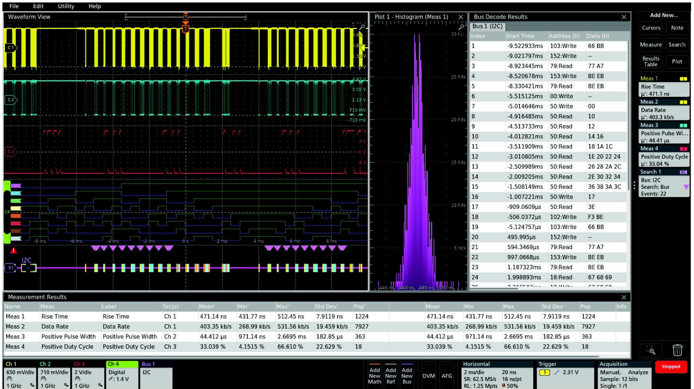
Viewing three analog channels, eight digital channels, a decoded serial bus waveform, decoded serial packet results table, four measurements, a measurement histogram, measurements results table with statistics and a search on serial bus events - simultaneously!
