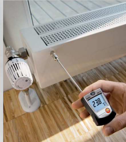
Surface temperature measurement on a radiator
