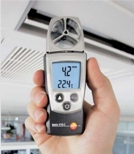
Flow velocity measurement at a duct outlet with 40mm vane
