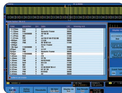
► Packet decode table showing decoded Identifier, DLC, Data and CRC for every CAN packet in a long acquisition.
